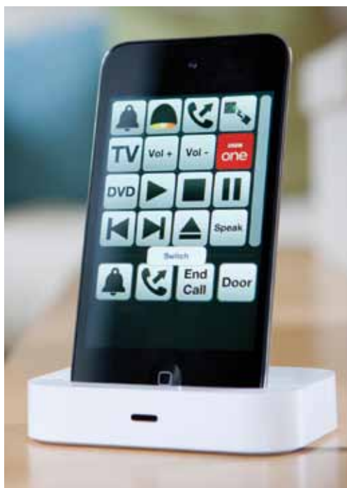
EvoAssist, developed by RSL Steeper, turns an iPhone into an environmental controller
