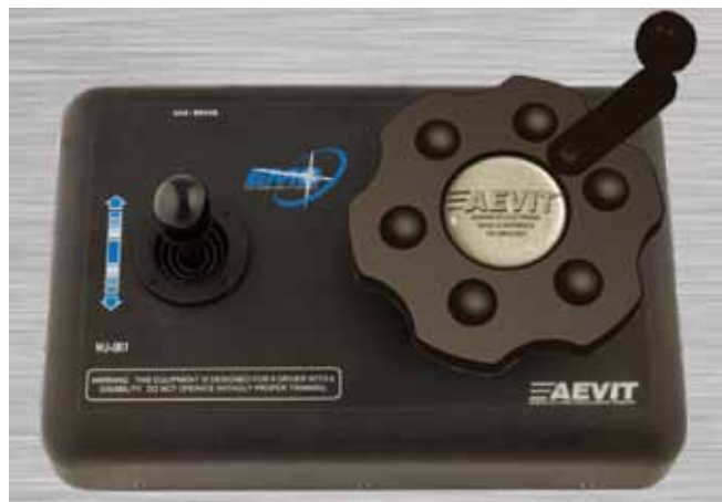
The EMC system with electronic gas and brake on the left and a mini steering wheel on the right
