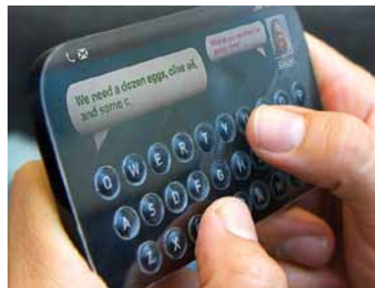
The Tactus Technology buttons are pumped up with a fluid
