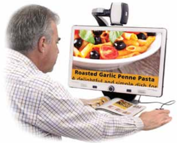
The DaVinci 3-in-1 magnifier turns text into speech output
